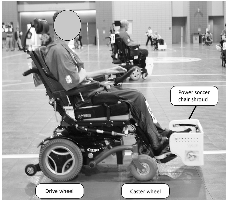
Figure 8. Electric powered wheelchair modified for soccer.
