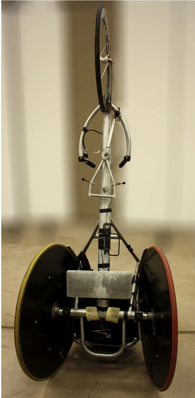
Figure 6. Racing wheelchair viewed from the bottom to show the T shape of the frame.
